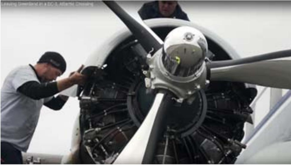
The only mechanical issues encountered came when they attempted to start-up the engines at the dawn of day two, taking off from Greenland. The Pratt and Whitney engines of the DC3 are normally very robust and stable; they have two banks of seven cylinders arranged in rings around the central crankshaft, generating 1,350HP from each engine. On this occasion the fuel-pump booster was set a little too
