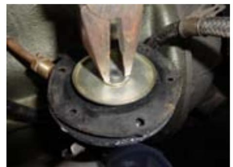
To remove the operating valves you have to remove the two screws that hold the retainer in position (shaped like a slightly bowed H) and the valves are now free to be withdrawn. Below the valves sits a figure 8 paper gasket.
