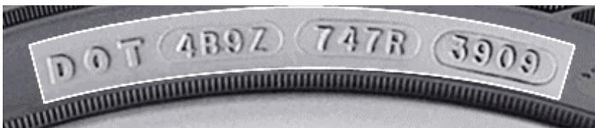
If the code has four digits, the tyre was made since the year 2000. That's a good start. This one was made in the 39<sup>th</sup> week of 2009; the tyre is 10 years old. A code of (0518) would indicate the fifth week of 2018, and so on.
